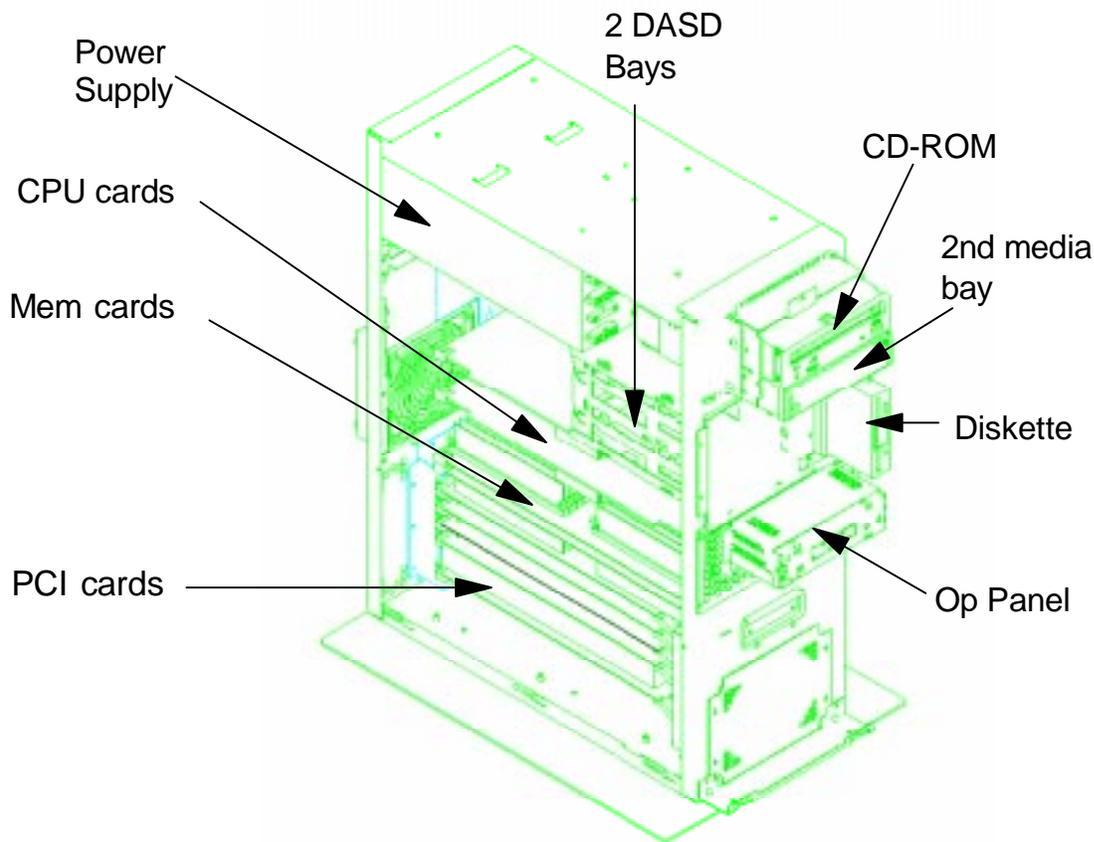
Figure 2. Model 260 Mechanical Package Layout
