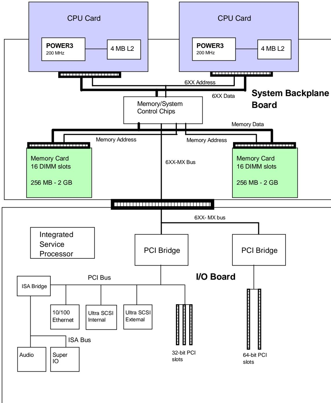
Figure 1. Model 260 Functional Block Diagram
