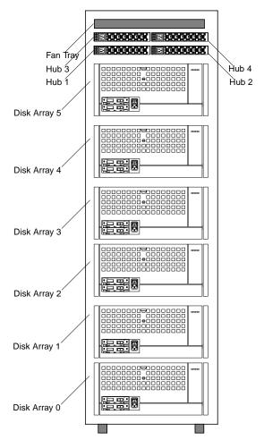
Figure 13. Rackmounting the Sun StorEdge A5X00 system
