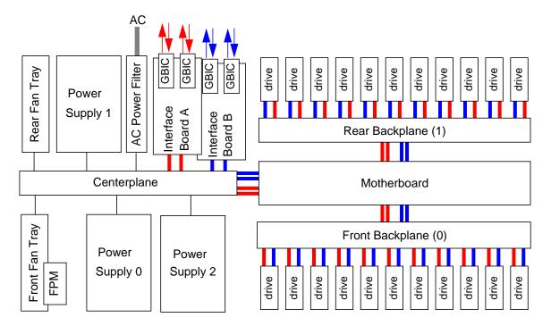
**Figure 4.** System architecture for the 22-drive configuration of the Sun StorEdge A5500 array. The 14-drive enclosure (Sun StorEdge A5100 array) places seven drives on each backplane.
