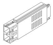
Figure 12. Gigabit interface converter (GBIC)
