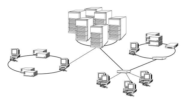
Figure 3. FC-AL's loop topology can support both simple and complex configurations
