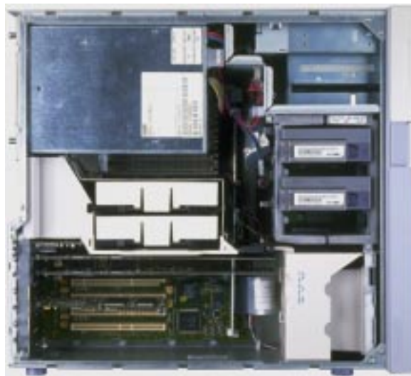
Figure 3. Ultra 60 workstation chassis with access panel removed, provides full access to internal options
